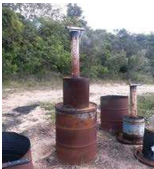
Figura 02 - Reator artesanal TLUD ( Top-Lid Updraft Gasifier )
