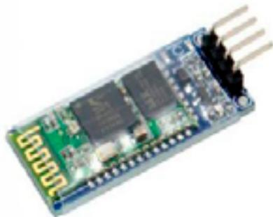
**Figura 4** - Módulo Bluetooth HC-06. **Fonte:** [https://www.usinainfo.com.br/bluetooth-arduino/modulo-bluetooth-hc-06-arduino-slave2826.html?search\\_query=bluetooth+HC-06+&results=6](https://www.usinainfo.com.br/bluetooth-arduino/modulo-bluetooth-hc-06-arduino-slave2826.html?search_query=bluetooth+HC-06+&results=6)
